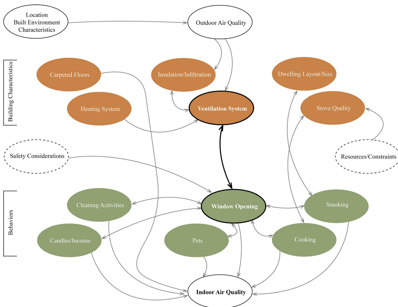
FIGURE 4 A diagram based on SES and Figure 1 representing the review findings regarding the indoor behavioral and physical (building characteristics) determinants of IAQ in dwellings and their interactions
