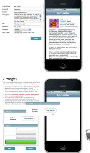
Figure 3. Screenshots of mobile application creation from the website. Information entered in the html fields on the left automatically appears on a replica iPhone screen (top). An author can drag and drop widgets from a predefined set onto replica iPhone screen to design one's own application (bottom).
