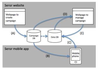
Figure 2. Functional architecture of Sensr; (a) campaign schema is saved to a server; (b) campaign schema retrieved to a mobile app; (c) reported data transfer between a server and a mobile app; (d) data retrieved to a web page; (e) discussion data saved to a server
